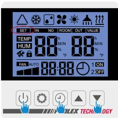
Press **+** + **+** + **-** simultaneously for 3s and the **SET** LED will flash quickly, indicating the control box is ready to be paired.
